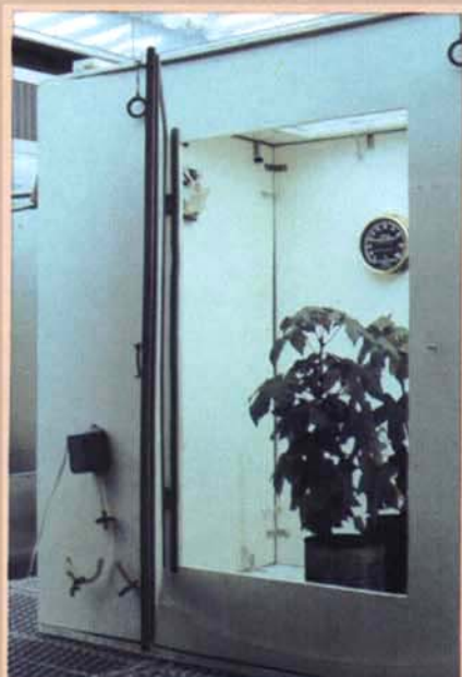
Fig. 1. A humidity cabinet inside a growth chamber provides equilibrium conditions for maintaining constant plant water potentials through an incubation period.
