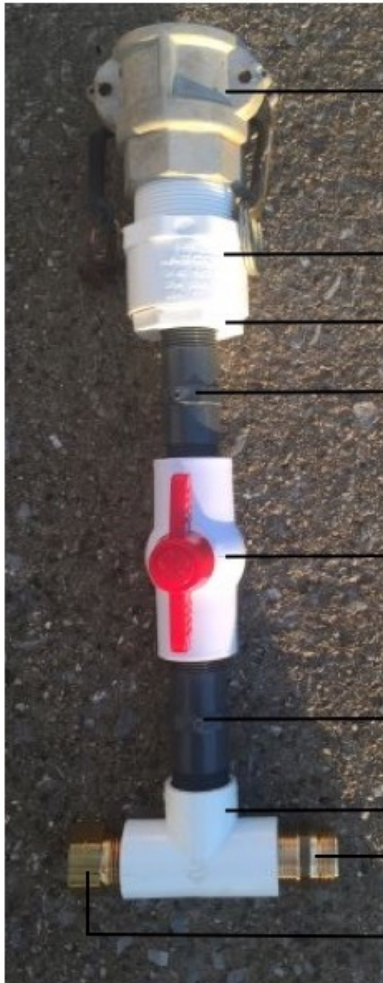
Figure 2. Manifold for injecting fertilizer into a \frac{3}{4} " water line (assumes legal backflow preventer elsewhere in the line)
