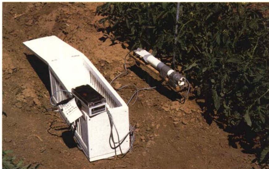
Fig. 1. The computerized air temperature and leaf wetness recorder (Model DP 223, Omnidata International, Inc., Logan, UT) used in the TOM-CAST forecasting system.
