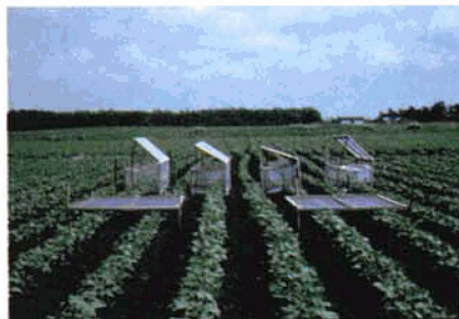
Fig. 10. Modification of the environment with polyethylene shelters and inert fiberglass screens. The shelters were used to shield bean plants from rain; the screens were used to decrease the momentum of raindrops as they passed through the screen and dripped onto the plants.
