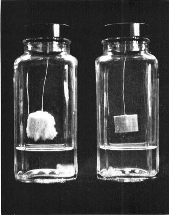
Fig. 4. A sample of clear wood, Acer saccharum , (right) and decayed wood (left) inoculated with Pholiota sp. and incubated for 6 weeks. The fungus grew on the clear wood sample, and mycelial bits that fell into the water also grew, but the sample was not decayed. The sample of decayed wood was decayed further.
