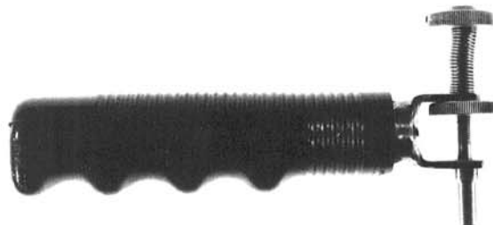
Fig. 7. Close-up of the single-pellet soil-sampler, \times 0.70 .
