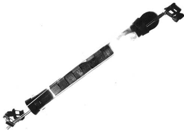
Fig. 2. Apparatus used to gas-sterilize wood decay test blocks. The glass cylinder is sealed at each end and the blocks are undergoing gas treatment.
