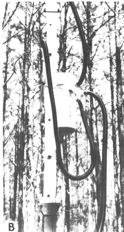
Fig. 1. Aspiration system for meteorological sensors used in plant epidemiology. A , The micrometeorological tower with the aspiration system in operation at three levels. B , The motor-driven aspiration system with attached sump hoses mounted on the tower. C , The complete aspiration system for one level. Arrow 1 indicates the Campbell CR-21 Micrologger. Arrow 2 indicates an aspirated, solar radiation-shielded sensor. D , The motor mounted inside the 20.3-cm (8-inch) ID PVC pipe viewed from the bottom. E , The motor mounting system. F , A cutaway view of the shielded relative humidity sensor.
