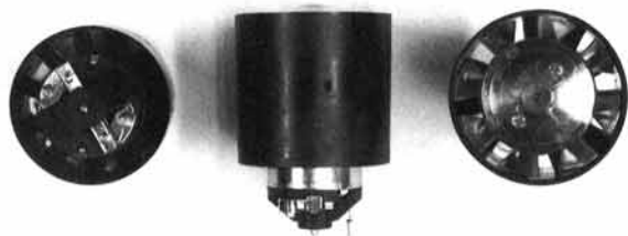
Fig. 7. Bottom, side, and top view of turbine blower and motor. The motor is of the type normally found in small hair dryers. The motor will operate on either AC or DC power, depending on whether or not a rectifier is included in the circuit.
