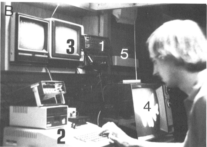
Fig. 3. Analysis of remotely recorded video images for estimating disease severity. A. Operation of hand-held portable color video camera focused on a group of four to six leaves with a black velvet tarp as a background. Images are shown recorded on a portable video cassette recorder. B. Analysis of recorded images stored on video tape (1) linked to the Apple II Plus computer (2) and a video monitor (3). Analyzed data or false-color representation of pixel intensity are displayed on another video monitor (4) or results of individual measurements are printed (5).
