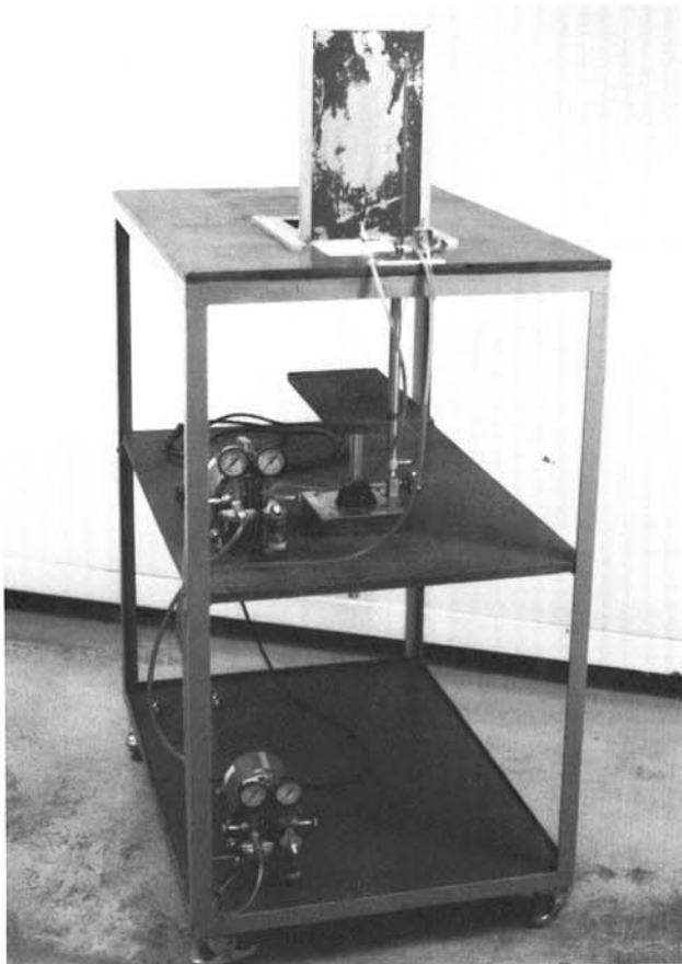
Fig. 2. Device for uniform deposition of liquid-suspended urediospores on cereal plant parts, mounted on a cart with locking wheels.
