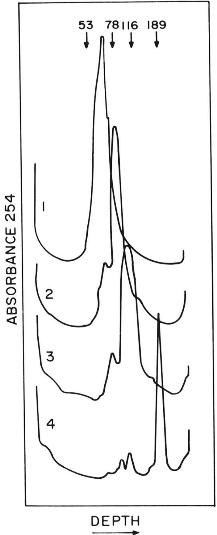
Fig. 3. Absorbance profiles of fractionated rate-zonal sucrose density gradients. The four MStpV nucleoprotein components were separated by one cycle of rate-zonal sucrose density gradient centrifugation in the SW 28 rotor. Each component was then pelleted by ultracentrifugation and re-centrifuged on rate-zonal sucrose gradients in the Beckman SW 50.1 rotor for 1.5 hr at 243,000 g (max.). Markers are TYMV top and bottom components (53 and 116 S, respectively), BMV (78 S), and TMV (189 S).
