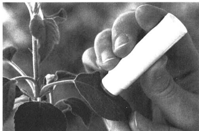
Fig. 2. Spores are sampled in the field by uncapping the sampler, extending the agar core 1–2 mm, and pressing its face against a foliar lesion. Spores adhere to the exposed, moist agar surface. The sampler is then capped for transport.
