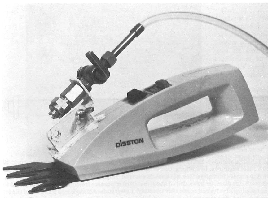
Fig. 2. Nozzle assembly mounted on a cordless electric grass clipper. Inoculum is transported from a pressurized tank to the nozzle, which atomizes it onto the clipper blades.
