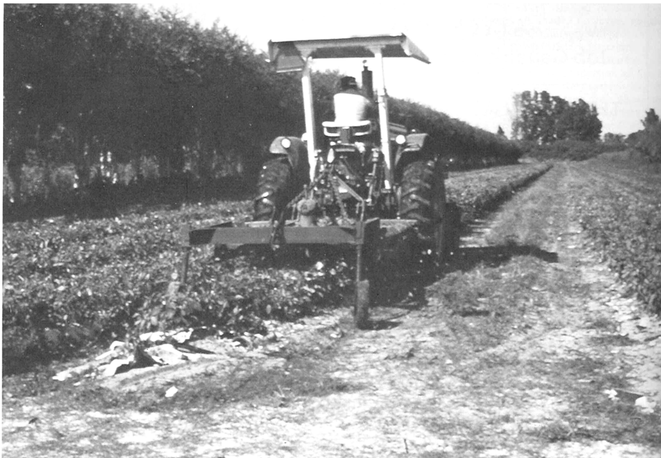
Fig. 1. Rotary mowing machine cutting back pepper plants in Florida. A second crop of fruit is produced on the regrowth.
