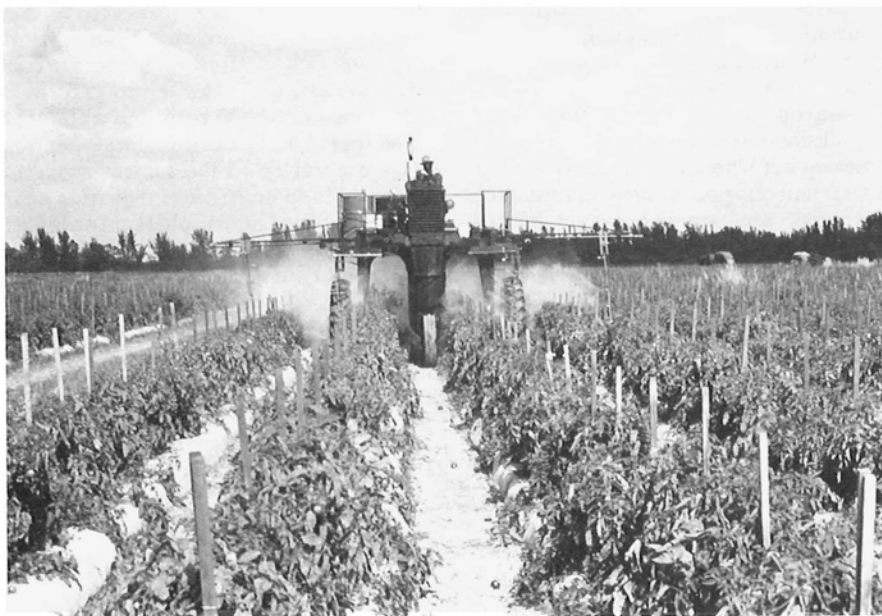
Fig. 2. High-clearance spray machine applying oil on stake tomatoes in Florida.
