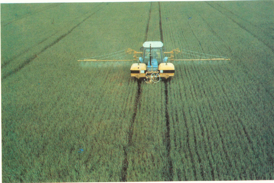
Fig. 2. Wheelways or "tramlines" being made in wheat to facilitate application of chemicals. (Courtesy Chafer of Doncaster)
