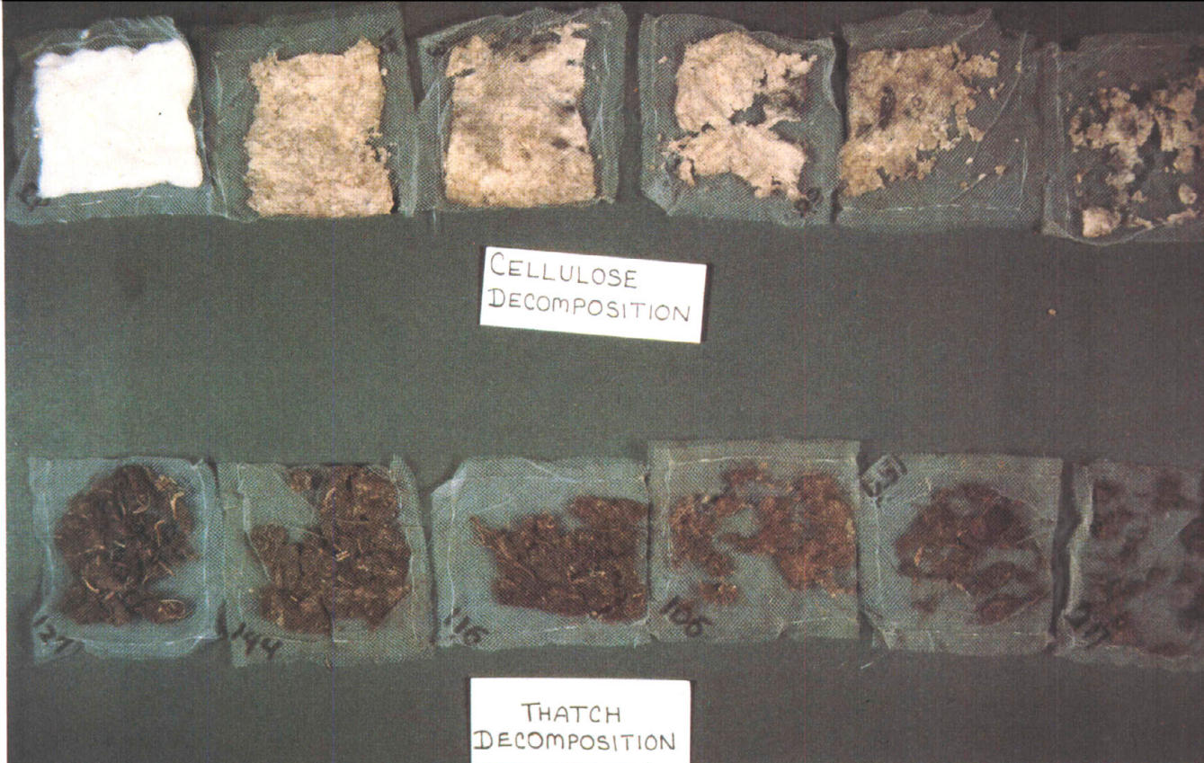
Fig. 5. Decomposition range for cellulose (cotton) and thatch buried in nylon-mesh bags for 5 months in turf plots treated with different fungicides; fresh bags are at left.
