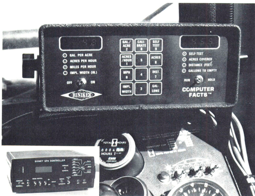
Fig. 4. Spray rate monitor with speed and flow rate sensors. (Inset) Controller.
