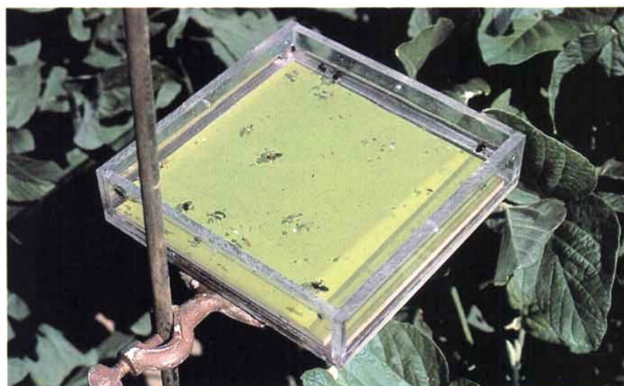
Fig. 2. The horizontal ermine lime (HEL) trap developed by INTSOY to monitor aphids and other insects visiting soybean fields.
