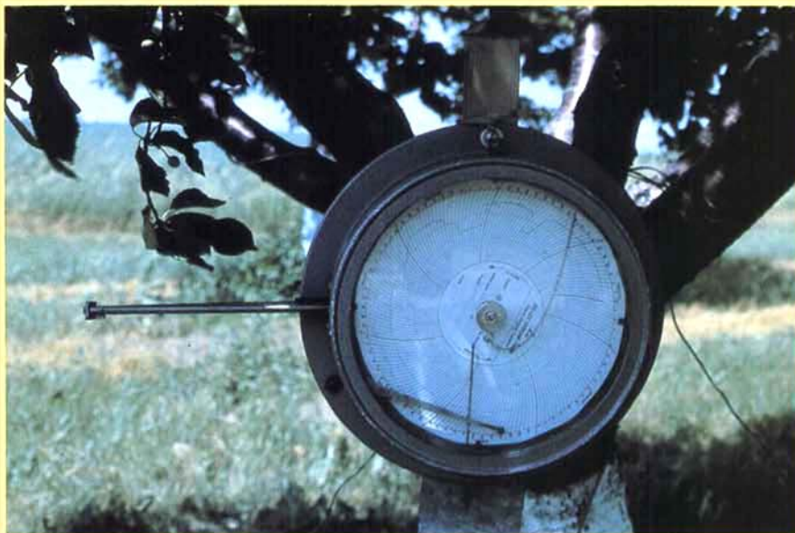
Fig. 2. DeWit leaf wetness meter for monitoring wet periods in alarm system for apple scab.
