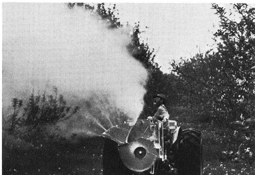
Fig. 4. Tractor-driven duster applying fungicides during rain after prediction of apple scab infection.
