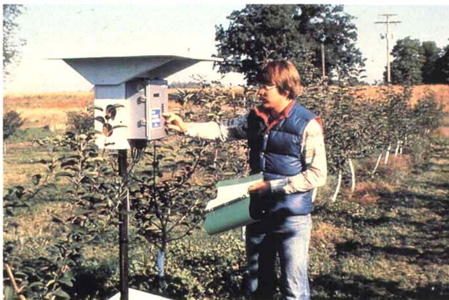
Fig. 8. Microcomputer in apple orchard is programmed to identify apple scab infection periods and to time fungicide sprays.
