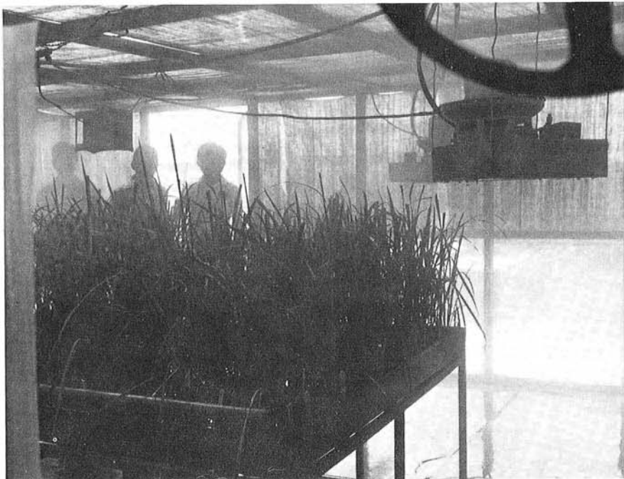
Rice plants are artificially inoculated with blast fungus in a specially constructed high-humidity chamber (top) that maintains free water on the leaves. (Bottom) Fogging device inside the chamber.
