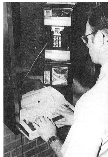
Fig. 2. A portable terminal can be used with a public phone.
