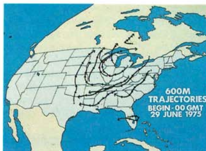
Fig. 3. Meteorological model showing movement of pollutant-containing air parcel across central United States into Minnesota on 29 June 1975. Air parcel's path was determined with weather-sounding data collected 600 m above the ground at various locations in the United States. Arrows indicate air parcel location at 12-hour intervals, starting at 0.00 hour Greenwich mean time (GMT).
