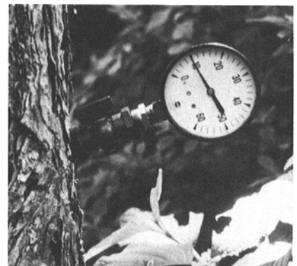
Fig. 1. Gauge cock and gauge mounted on an elm stem showing an internal wetwood gas pressure of 0.7 kg/cm 2 .
