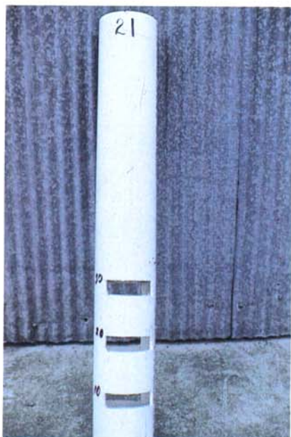
Fig. 7. Plastic tube used to demonstrate migration of trichodorids after soil fumigation. The tube was filled with sterilized field soil, a potato plant was planted in the tube, and the tube was placed into soil previously treated with 1,3D.
