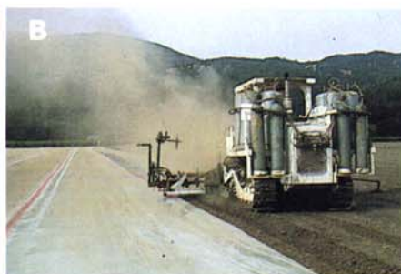
Fig. 7. Deep placement of (A) 1,3-D and (B) methyl bromide under polyethylene cover.
