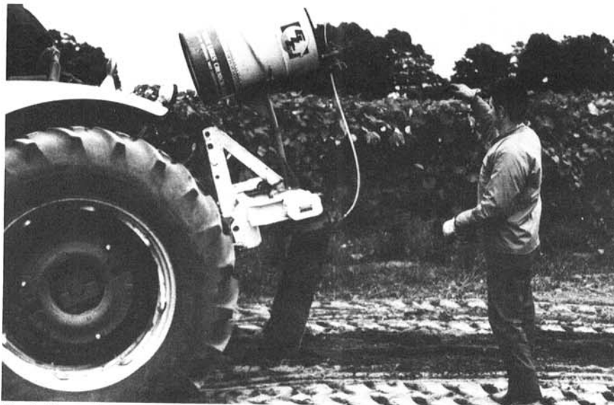
Fig. 1. Deep-placement soil fumigation shank, which fits on a three-point hitch of a large (90-hp) tractor.
