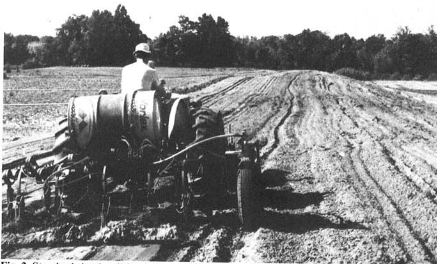
Fig. 2. Standard shank soil fumigator used for shallow placement of soil fumigants.
