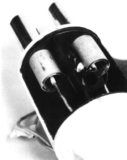
Fig. 4. Portion of a ventilated psychrometer for monitoring relative humidity.
