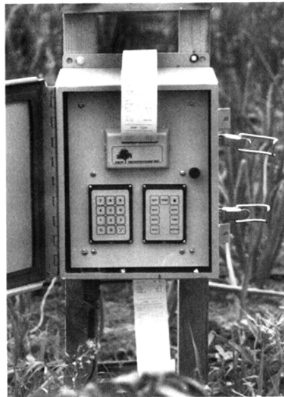
Fig. 14. Programmable data logger with two input channels and data printout (Crop Technologies Inc., Waterloo, Ontario, Canada N2J 3X2).
