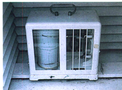
Fig. 3. Hygrothermograph for monitoring air temperature and relative humidity, positioned in an instrument shelter.
