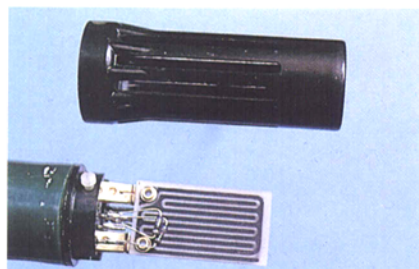
Fig. 5. (Bottom) Humidity sensor constructed from a sulfonated polystyrene plate to which two electrodes are bonded, and (top) a protective cover (Phys-Chemical Corp.).
