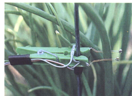
Fig. 8. Electrical wetness sensors clipped onto a green onion leaf.
