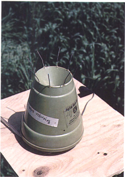
Fig. 10. Tipping-bucket rain gauges manufactured by (top) Weathertronics Inc., Sacramento, CA 95841, and (bottom) Edmund Scientific Co., Barrington, NJ 08007; wires have been added to discourage birds from roosting on the gauge.
