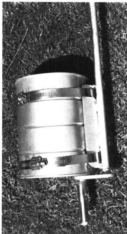
Fig. 1. Probe used for collecting 1-cm-diameter by 8-cm-long cores of turf and soil during nematode sampling.
