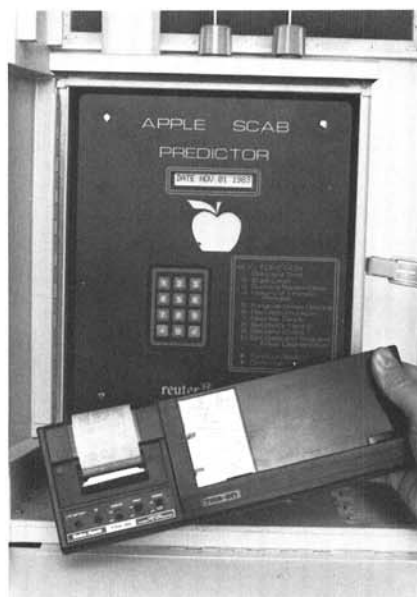
Fig. 4. Apple scab predictor with plug-in printer for obtaining permanent copies of predictions and weather data.
