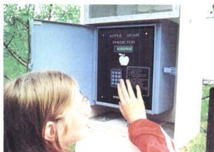
Fig. 1. A Reuter-Stokes apple scab predictor (left) in the field and (right) being checked to determine if infection has occurred.
