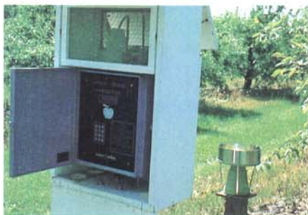
Fig. 1. A Reuter-Stokes apple scab predictor (left) in the field and (right) being checked to determine if infection has occurred.
