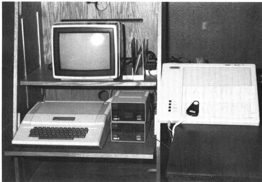
Fig. 2. APPLE II PLUS microcomputer system with digitizing board to read hygrothermograph charts.
