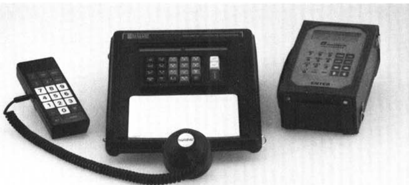
Fig. 1. Commonly available electronic notebooks (left to right): Norand Sprint 100, Datamyte 1000, and Omnidata Polycorder.
