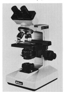
sophisticated optical and illumination systems needed for phase-contrast photomicrography and oil-immersion techniques, the Alphaphot-Kt uses the Koehler illuminator to provide ample light output from a 20-W quartz-halogen, low-voltage source. The field diaphragm, which can be centered, is imaged on the specimen to maximize contrast.
