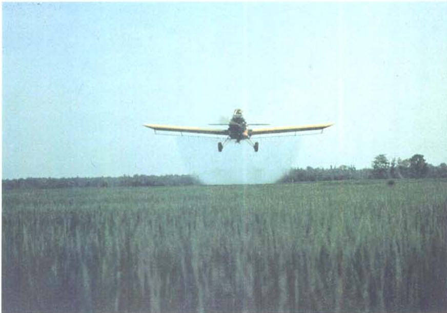
Fig. 3. Aerial application of Collego to rice. C. gloeosporioides is normally applied aerially with standard agricultural equipment at a rate of 10 gal/acre (94 L/ha) containing 2 \times 10^6 spores per milliliter.
