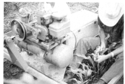
Fig. 4. Rig for two-row airbrush inoculation of plants in the field.
