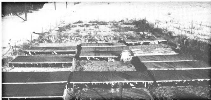
Fig. 1. Field plot in 1984. Half of the treatments were exposed to solar radiation and half were shaded by enclosing them under black polyethylene tents.
