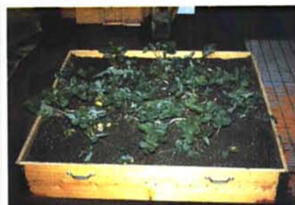
Fig. 8. Experimental setup of strawberry plant canopy consists of two circular "rows" 30 cm apart. Entire 1.2 \times 1.2 m area is impacted by a uniform generated rain.
