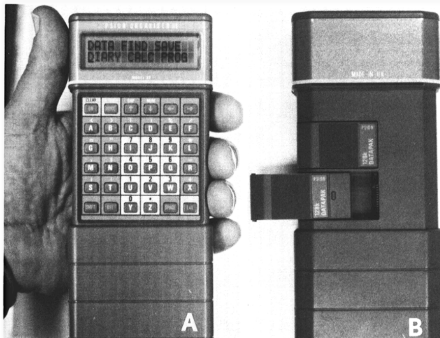
Fig. 1. (A) The compact Organiser II-XP has a two-line display and an alphanumeric keypad. (B) Two slots on the back of the Organiser accept Datapaks and Ram Paks for permanent storage of data.
