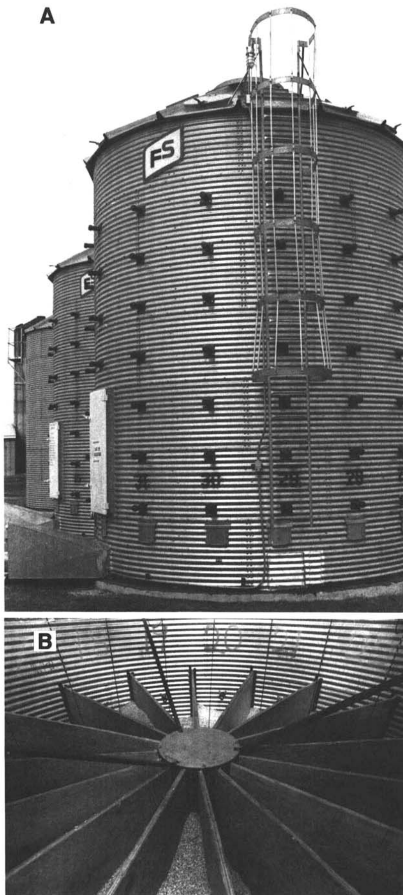
Fig. 1. Experimental bin with sampling ports that allow for samples to be taken from various grain depths. The 16 wedge-shaped compartments in the bin accommodate various experimental treatments.
