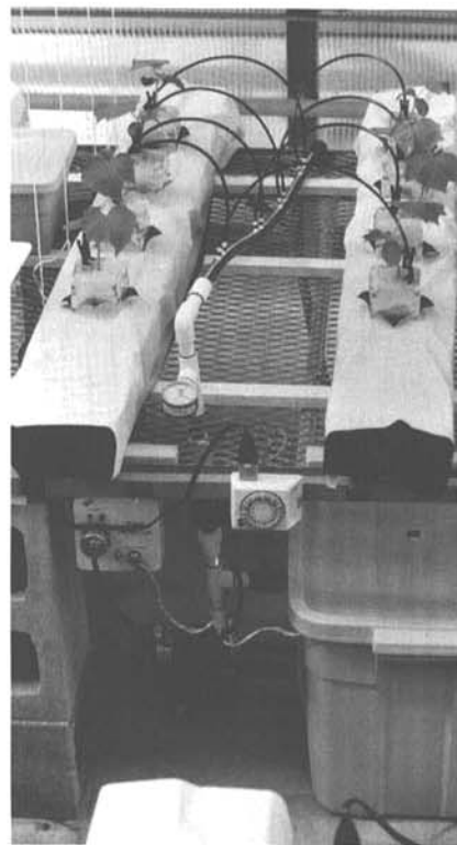
Fig. 2. Photograph of an individual recirculating hydroponic unit. Two rock wool slabs, each containing four cucumber plants, were connected to a reservoir containing 50 liters of nutrient solution.
